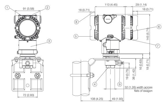
1 Adjustments | 2 Identification plate | 3 Certification plate | 4 Process connection | 5 Terminal side | 6 Integral display housing | 7 Electronic side | 8 Space for cover removal | 9 Drain/vent valve
