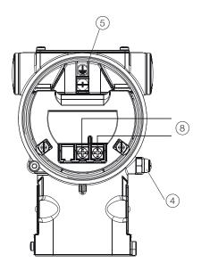
1 Power source | 2 Remote indicator | 3 Handheld communicator | 4 External ground termination point | 5 Internal ground termination point | 6 Line load | 7 Harting Han 8D socket insert for mating plug (supplied loose) | 8 Fieldbus line (polarity independent)
